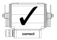
The number of plates changed rotated through 180° must be the same at both ends of the shaft, i.e. they must be symmetrical. (See Fig.) The unbalance plates can also be removed for fine adjustment, they must then be replaced by spacer discs. The centrifugal force is reduced by turning the unbalance plates through 180° at both ends.
