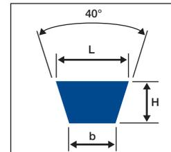
A V belt is driven by its sides. The belt must come off its pulley by 1mm, so that the product conveyed may not touch the pulley.
