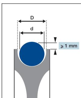
A round belt is driven by a round-groove pulley. The diameter of this round groove should be 1mm greater than the diameter of the belt for smaller round belts, and 2mm greater for round belts from diam. 12 mm on.
