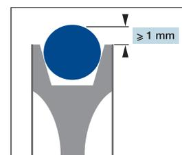
$d < 12 \text{ mm}$      $D = d + 1 \text{ mm}$
