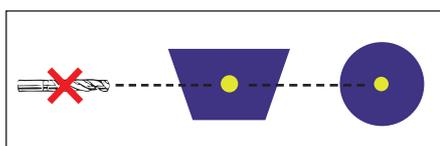
Our reinforced belts are welded in the same way as the other non-reinforced belts, **WITHOUT REMOVING THE REINFORCEMENT**. This avoids all the problems associated with drilling. Our special reinforcement does not fuse at the welding temperature of our thermostated irons (260°C). There is therefore no danger of contaminating the weld.
